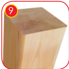
9 Soft conifer wood 140 x 140 mm, coreless, knotless, glued in layers with polyurethane glues, totally resistant to water. Wood posts processed in three-phased impregnation process.
