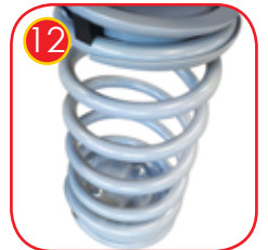
12 Springers' springs made of spring steel. The diameter of the spring is 200 mm and the diameter of the rod is 20 mm. The springs and the fastenings are galvanized and powder coated with polyester paint, UV resistant and QUALICOAT attested. The fastenings are designed especially for solutions used on a playground, so they are stripped of elements which can cause danger to children.
