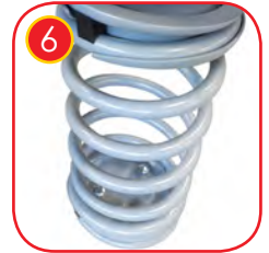
6 Springers' springs made of spring steel. The diameter of the spring is 200 mm and the diameter of the rod is 20 mm. The springs and the fastenings are galvanized and powder coated with polyester paint, UV resistant and QUALICOAT attested. The fastenings are designed especially for solutions used on a playground, so they are stripped of elements which can cause danger to children.
