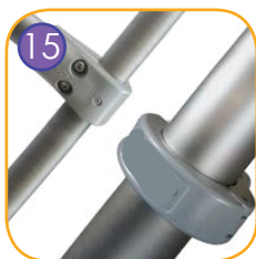
15 System of connectors and clamps made of strong aluminum alloy. Aluminum is secured by the process of electrophoresis and powder coating with polyester paint UV resistant and QUALICOAT attested.
