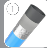
1 Solid construction made of black steel S235JR, cleaned in the sand-blasting process. Protected against corrosion by galvanizing and powder coating with polyester paint QUALICOAT attested.
