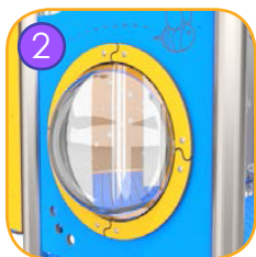
2 Hemispheric window with a diameter of 400 mm. Material: heat-formed polycarbonate 5 mm thick, resistant to vandalism.
