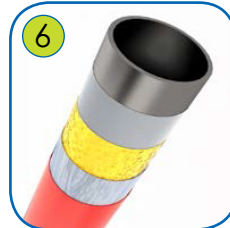
Solid construction made of black steel S235JR, cleaned in the sandblasting process. Protected against corrosion by galvanizing and powder coating with polyester paint QUALICOAT attested.
