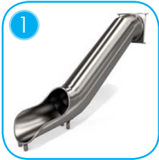
1 Tube slide made of stainless steel AISI 304. The metal sheet is 2 mm thick and the end section is finished with a band made of pipe 33.7 mm. The surface is polished.
