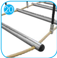
20 The passage module made of polypropylene rope with a diameter of 16 mm with a steel core and AISI204 stainless steel. Rope connections clamped in sleeves made of durable aluminum alloys.
