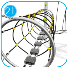
21 The passage module made of polypropylene rope with a diameter of 16 mm with a steel core, AISI204 stainless steel and HDPE plates. Rope connectors made of injection molded polyamide. Ends of ropes clamped in sleeves made of durable aluminum alloys.
