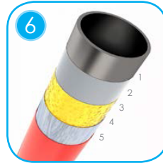
6 Solid construction made of black steel S235JR, cleaned in the sandblasting process. Protected against corrosion by galvanizing and powder coating with polyester paint QUALICOAT attested. 1 – steel, 2 – sandblasting, 3 – iron phosphatizing, 4 – zinc base, 5 – polyester powder paint.
